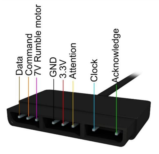
/JOYn are two separate signals (/JOY1 for left card/pad, /JOY2 for right card/pad) (whether it is an card or pad access depends on the first CMD bit). All other signals are exactly the same on all four connectors (except that pin8 and shield are missing on the card slots).
